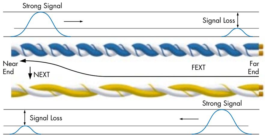
Noise occurring at the far end can be difficult to measure because much of the noise is lost or attenuated as it makes its way to the testing device. Therefore, it is common practice to “take out” the attenuation effects and look at the pure noise taking place. When looking at the noise minus the effects of attenuation, the term “Equal-Level Far-End Crosstalk,” or EL-FEXT, is used.
