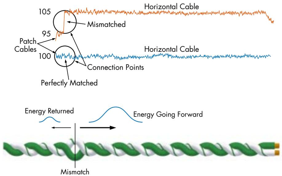
This mismatch will cause energy to reflect back starting at the point of discontinuity. Where impedance defines the potential of mismatch, **return loss** quantifies the consequence. Measured in dB returned signal, return loss helps to indicate how much signal will be lost due to reflected energy.
