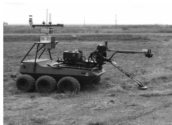
Figure 8: ARS Mounted on "Scout" Remotely Operated Vehicle
