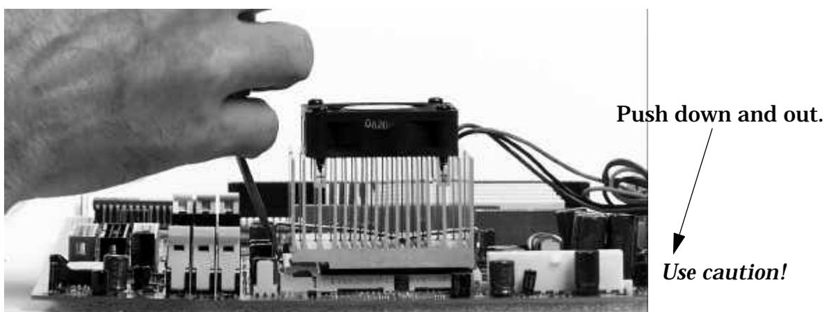
Figure 16. Pushing the Clip Past the Socket Lug
