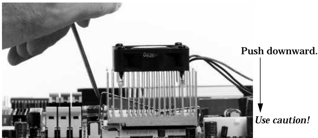
Figure 15. Pushing the Heatsink Clip Down
