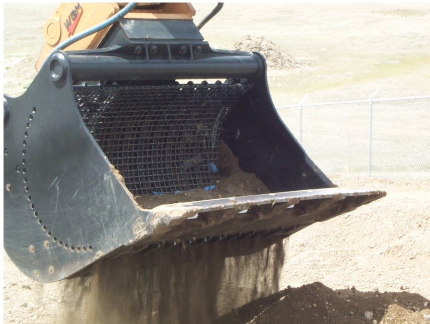
Figure 3. VRL-8 Sorting Bucket with Replaceable Screen
