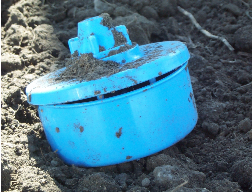
Figure 8. PMA-2 Plunger Removed and Lid Partially Removed By Rototiller
