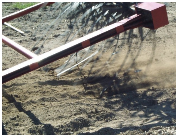
Figure 6. Aegis Flail “Tickling The Ground” Instead Of Slapping
