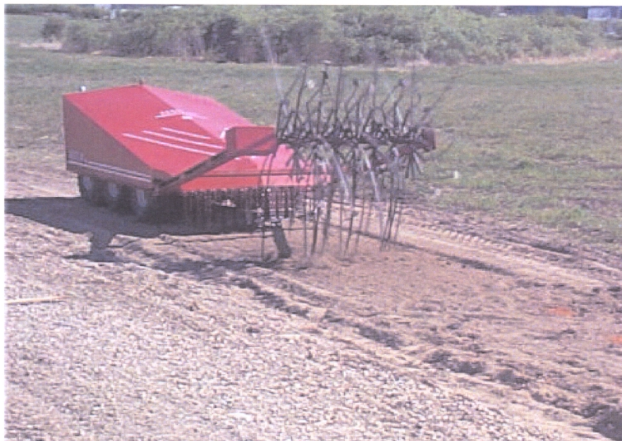
Figure 1. Omega 5 Flail Demining Implement.
