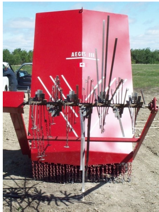
Figure 8. Omega 5 Aegis Mini-Flail With Most Slappers and Cutters Removed
