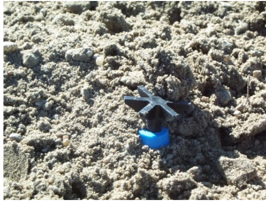
Figure 7. PMA-2 Missed By Aegis Mini-Flail Despite Being Exposed
