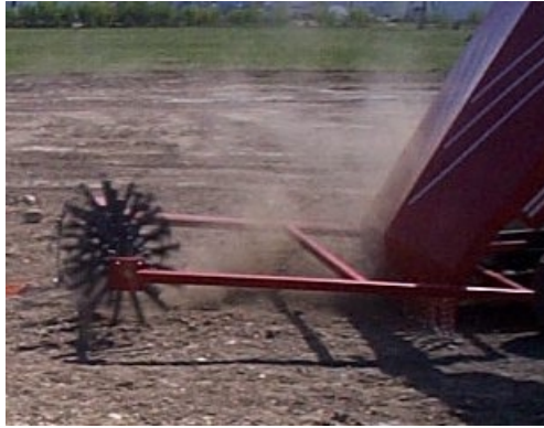
Figure 9. Aegis Mini-Flail Operating With Only Cutter Chains
