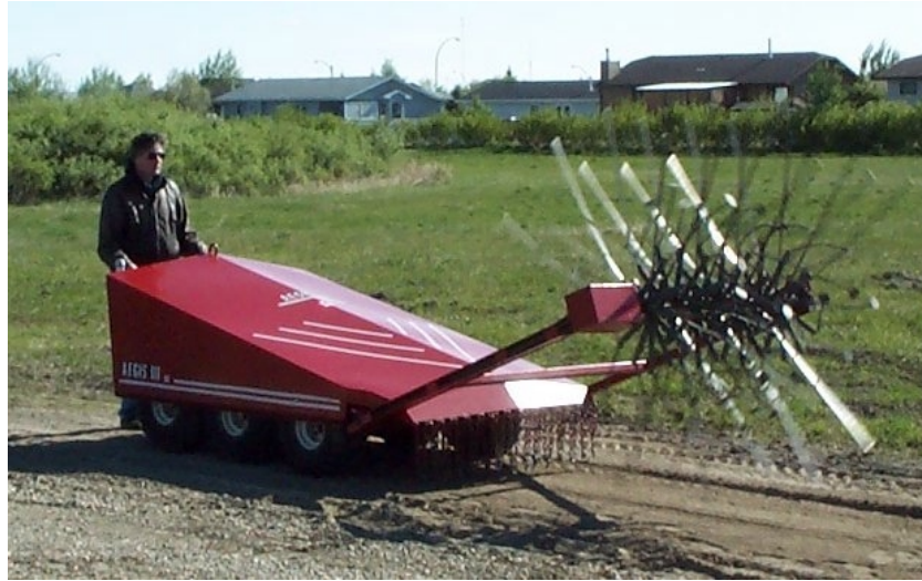
Figure 4. Omega 5 Aegis Flail Under Manual Control
