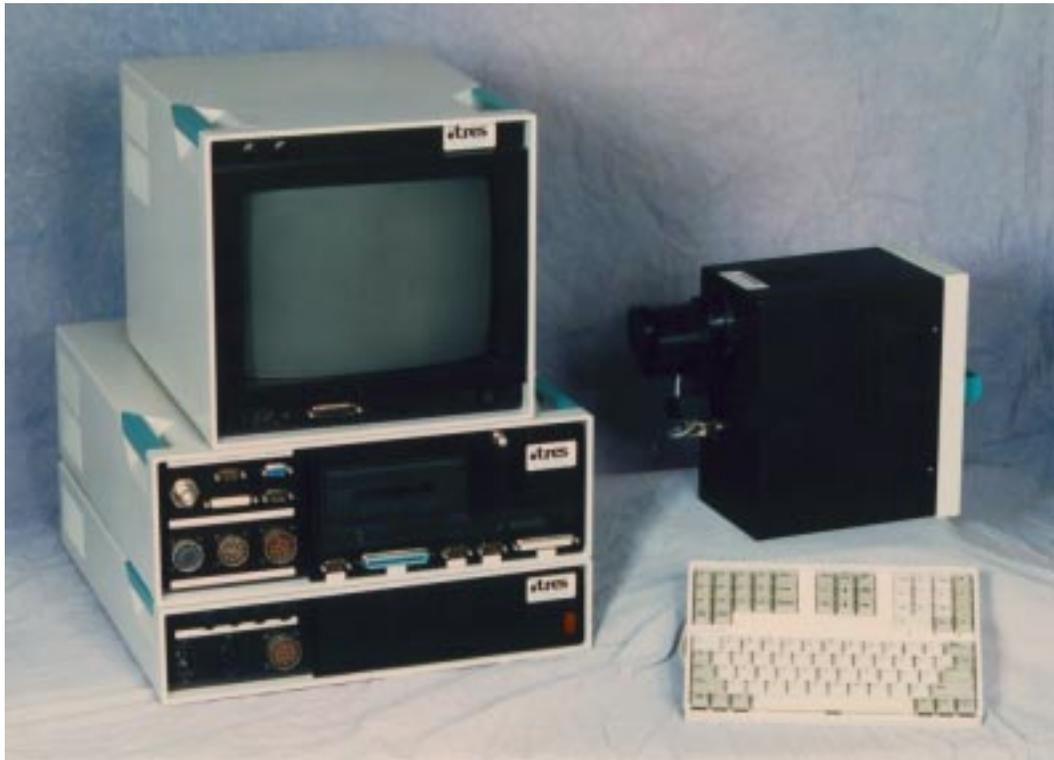
**Figure 1.** *casi* hyperspectral imager. At left from top to bottom are the monitor, control unit and power supply. At right rear is the sensor head.
