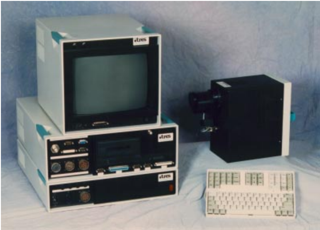
Figure 3. casi hyperspectral imager. At left from top to bottom are the monitor, control unit and power supply. At right rear is the sensor head.
