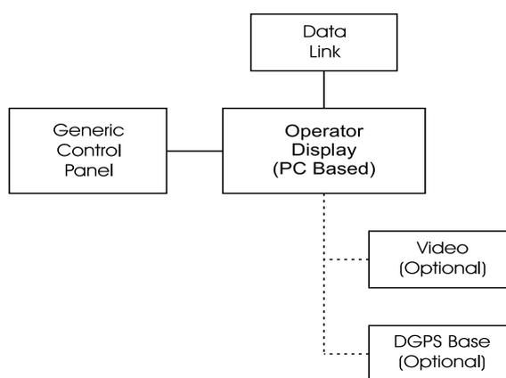
Figure 2: Operator Control Station Block Diagram
